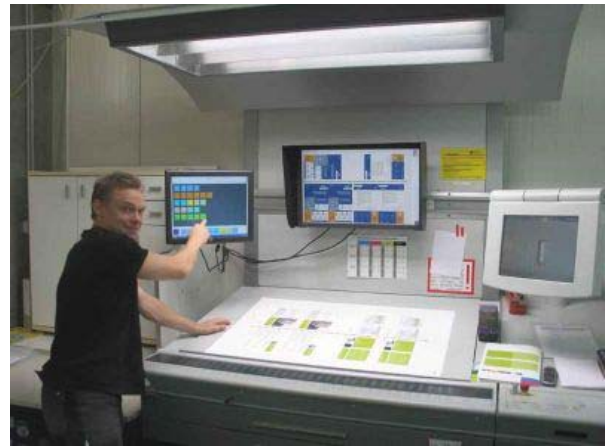
A Heidelberg Speedmaster operator checks print against proof with Veripress monitor and touch-screen control
