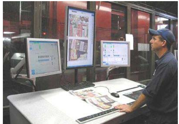
For newspaper and publication printing, the Veripress monitor is mounted in "portrait" orientation
